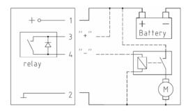
When connecting the relay contacts ensure correct polarity!
